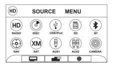
Touch the RADIO, DISC, USB/iPod, SD, BT, NAV, SAT, AUX1, AUX2 or CAMERA button to select the corresponding source.
